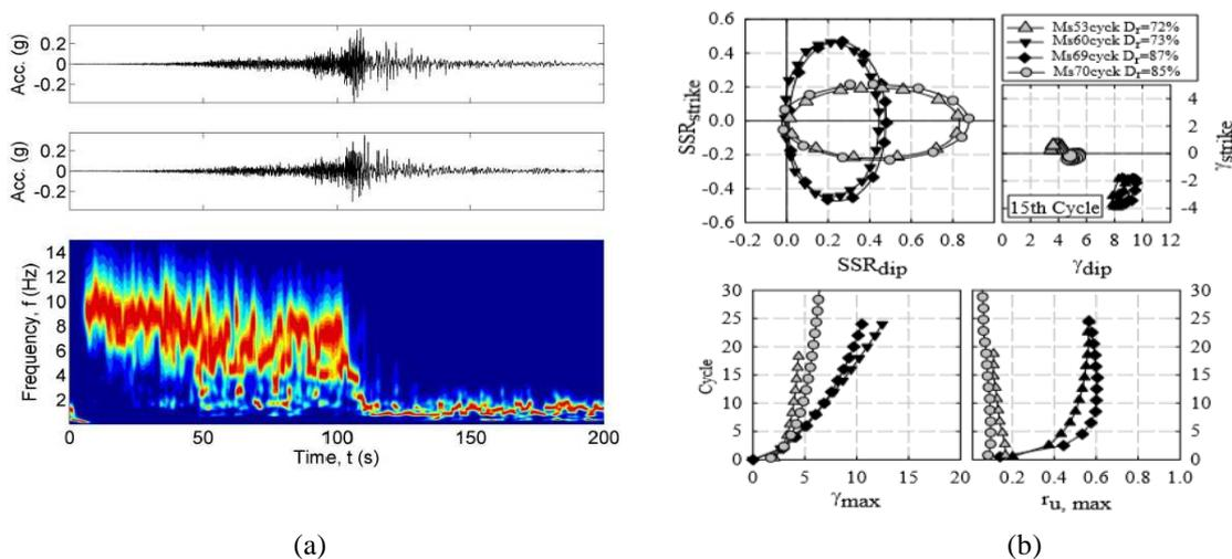
**Fig. 1.** Horizontal ground surface time histories (a) and normalized Stockwell spectrogram for IBR014 site in 2011 Tohoku earthquake (Kramer & Greenfield, 2019); (b) results of bi-directional simple shear tests (Kammerer et al. 2004)
