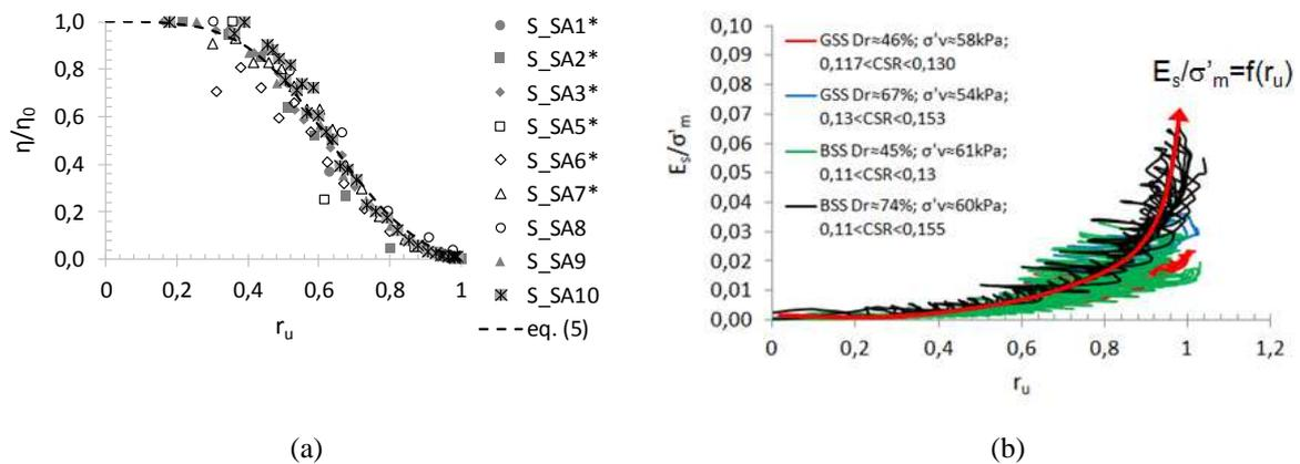
**Fig. 2.** Normalized apparent viscosity  $\eta/\eta_0$  (a) and normalized cumulative strain energy  $E_s/\sigma'_m$  (b) versus pore pressure ratio, measured in cyclic tests on saturated sandy soils (Lirer & Mele, 2019)
