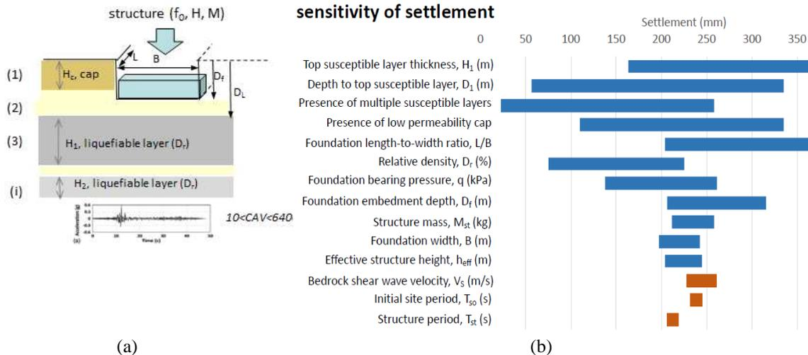
**Fig.5.** Results of 3D (a) numerical study: sensitivity (b) of average permanent foundation settlements to input parameters (Karimi et al., 2018)
