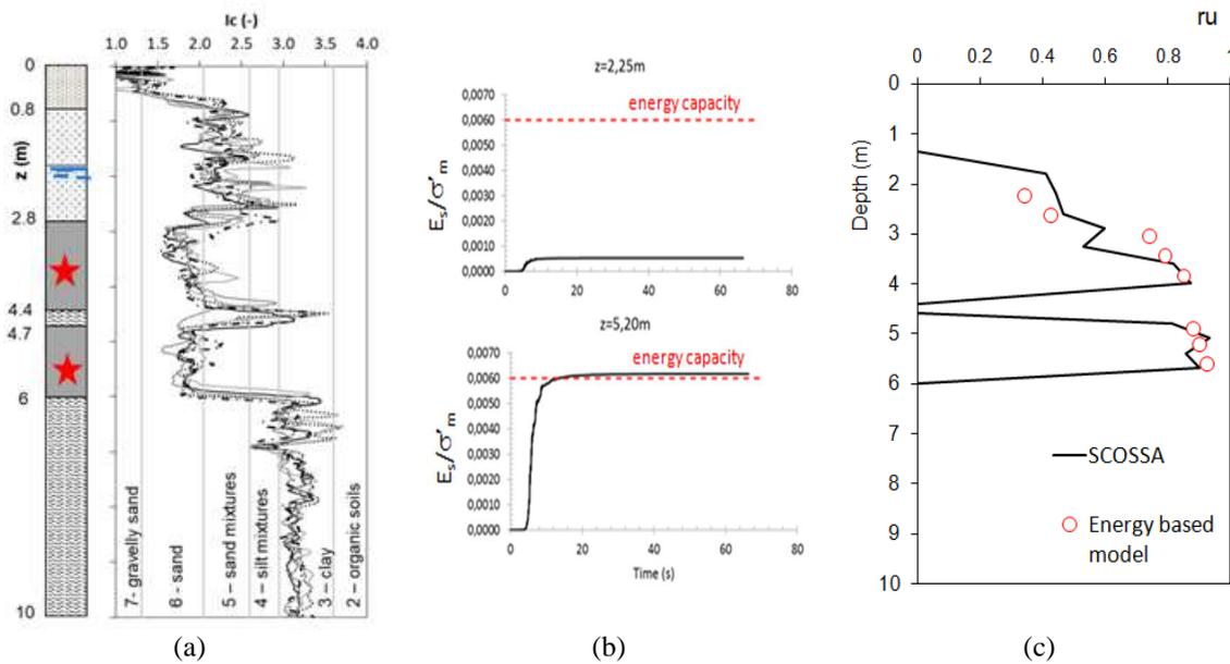
**Fig. 3:** Liquefaction potential analyses for the site of Pieve di Cento – trial field in LIQUEFACT project (a): comparison between pore pressure ratio computed via the simplified energy based analysis and via the 1D “loosely coupled” dynamic analysis (c)
